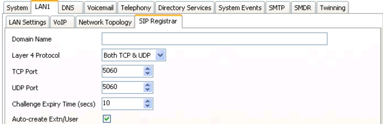
The screenshot shows the 'SIP Registrar' configuration window. The 'Auto-create Extn/User' checkbox is checked. Other settings include: Domain Name (empty), Layer 4 Protocol (Both TCP & UDP), TCP Port (5060), UDP Port (5060), and Challenge Expiry Time (secs) (10).
