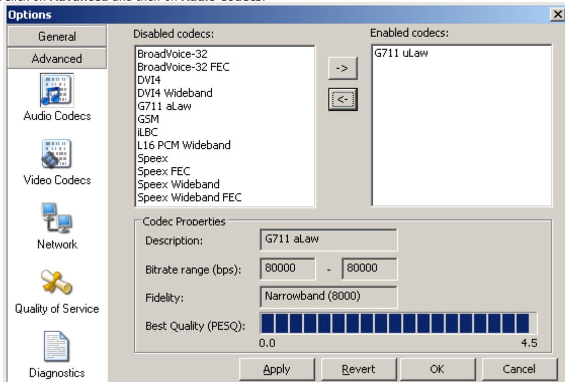
3. Ensure that the **Enabled codecs** column contains just a single codec. That codec must be one supported by the IP Office extension configuration for the SIP extension.
