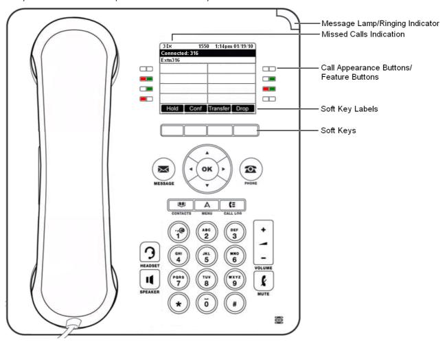
This phone supports 24 programmable call appearance/feature buttons. The labels for these buttons are visible on the main display and can be controlled by the adjacent buttons.
