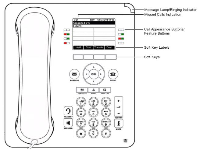
This phone supports 24 programmable call appearance/feature buttons. The labels for these buttons are visible on the main display and can be controlled by the adjacent buttons.
