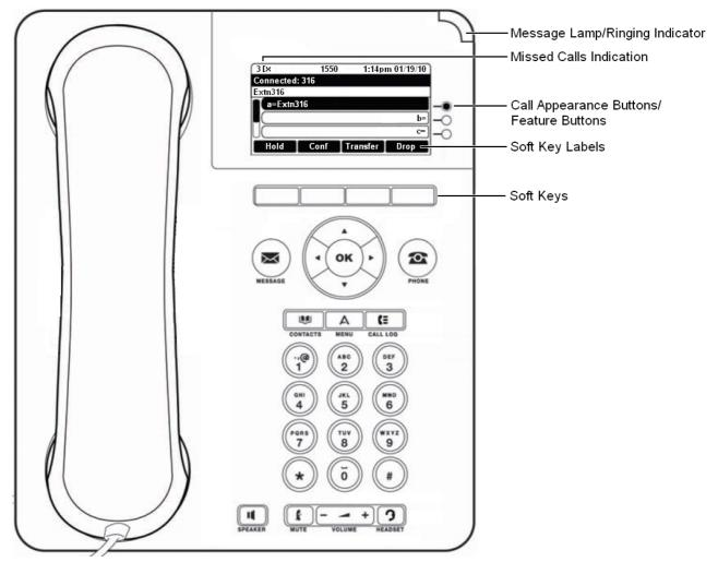
This phone supports 12 programmable call appearance/feature buttons. The labels for 3 of these buttons are visible on the main display and can be controlled by the adjacent buttons to the right. You can use the  $\blacktriangle$  up and down  $\bigtriangledown$  arrow keys to scroll the display. You can also use the  $\blacktriangleleft$  left and right  $\blacktriangleright$  arrow keys to move through the button features in pages of 3.
